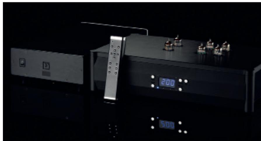
Nick Doshi says he was careful to avoid using exotic tubes in the circuit because he wanted to ensure that tube availability would never become an issue. There are three pairs of tubes: two 12AX7s in the first gain stage, two 12AU7s in the second stage as a parallel follower to drive the EQ section, and two 12DW7s for the final gain section and output driver. Because the circuit has no feedback, tube matching is important to maintain tight channel balance.
