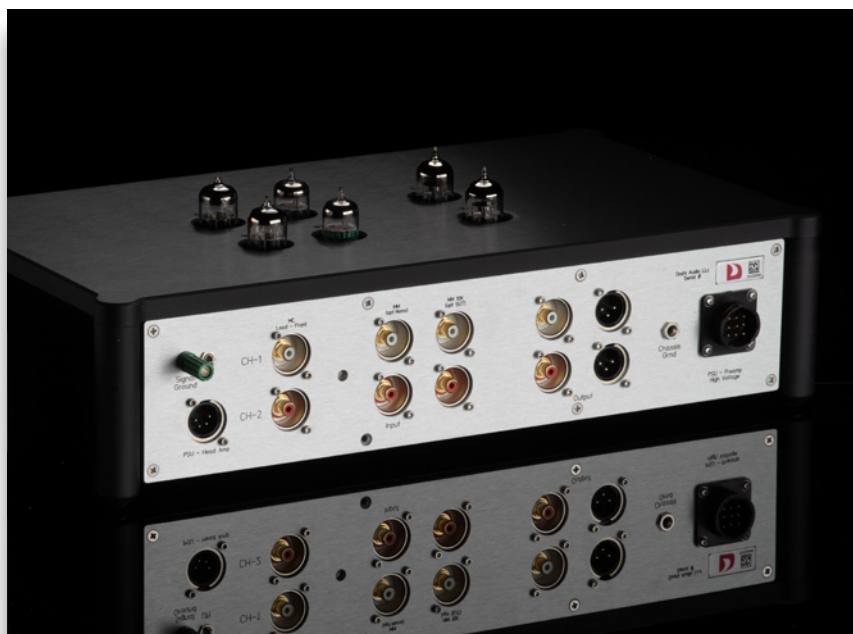
Rear panel showing inputs, outputs and PSU connections
