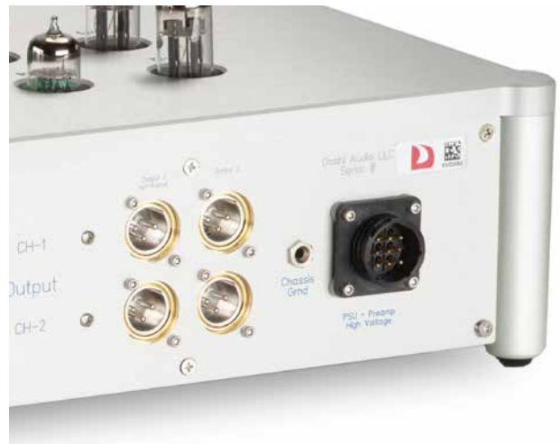
Rear of Audio unit showing output and HV power connection
