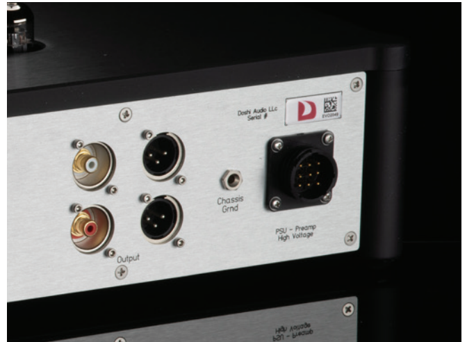
Rear of Audio unit showing output and HV power connection
