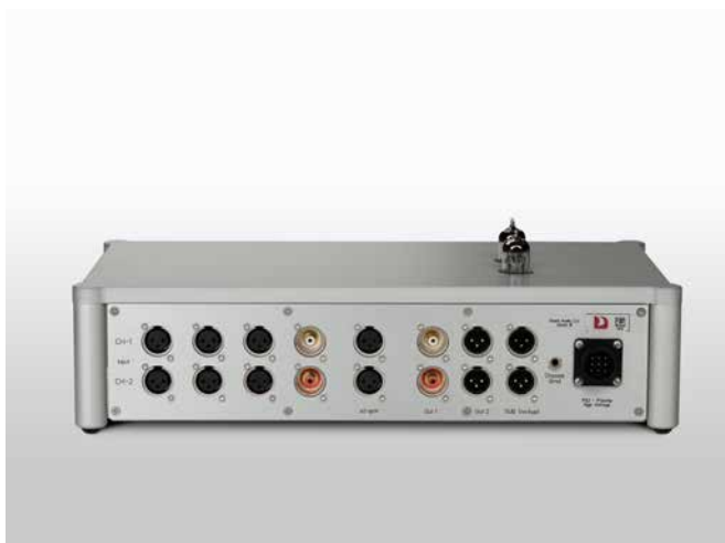
4 Inputs on the Left | 3 Sets of Outputs on Right Rear of Audio Unit and HV Power Connection
